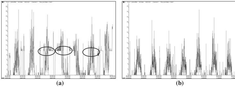
**Figure 5** Radcom trace showing; a) continuous flushing (circled) occurring intermittently in a washroom over a 7 day period; b) an example of a normal flushing regime
