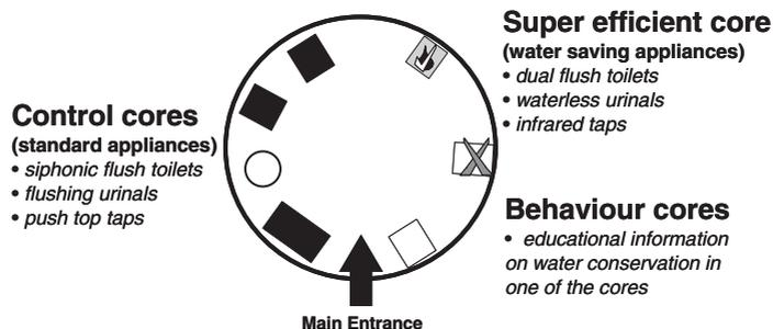
**Figure 2** Layout of the core buildings housing the washrooms within the Dome
