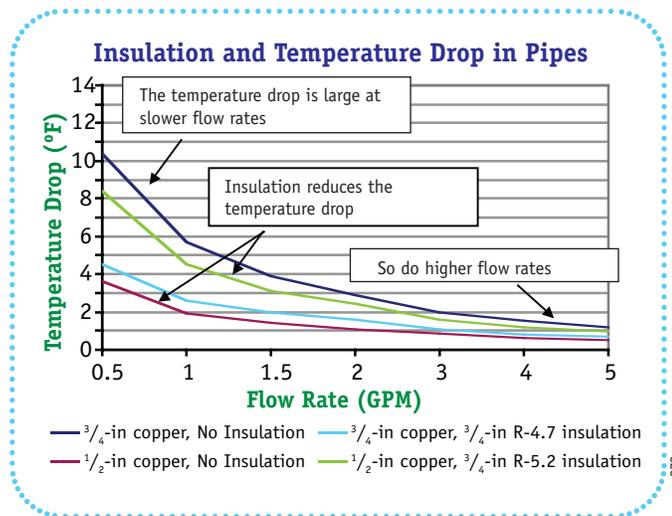
**Figure 1.** Based on tests of 1/2- and 3/4-inch piping for a given flow rate, R-4 insulation will reduce the temperature drop by half. The graph is for 100 ft of pipe. The hot water begins at 135°F and the ambient air temperature surrounding the pipes is 67°F.
