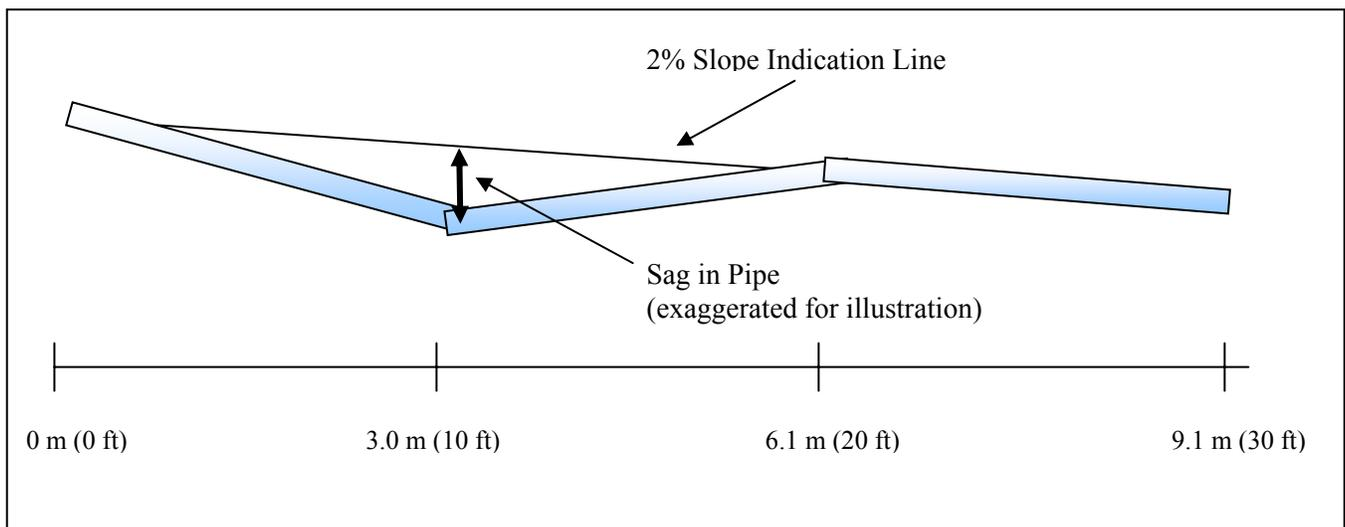
Figure 15a: Effects of Sag in Pipe Slope
