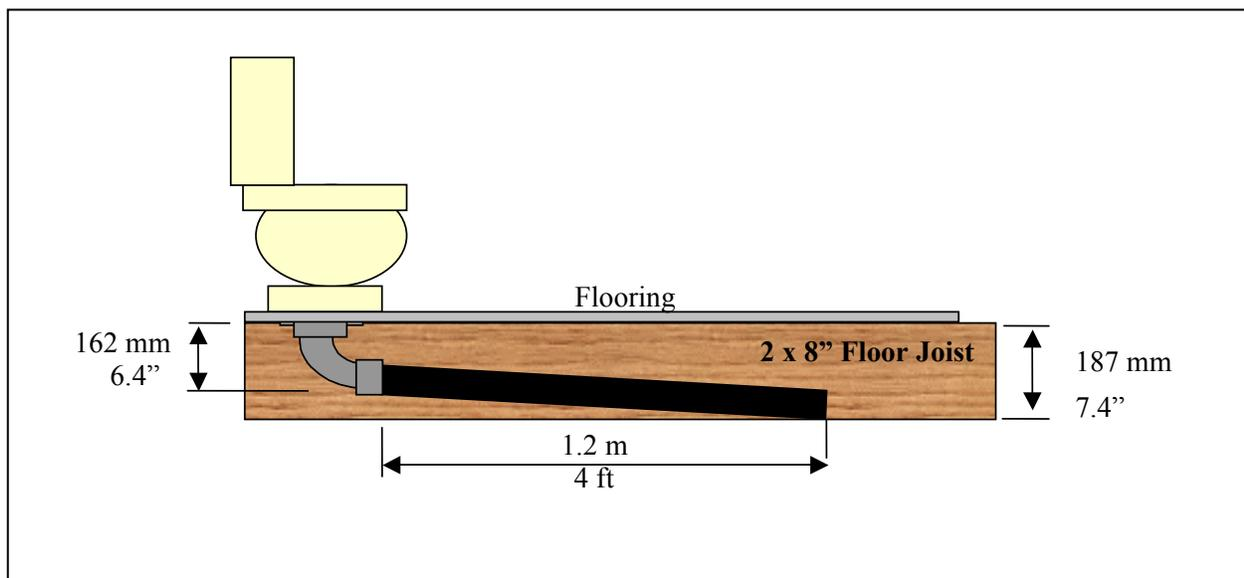
A 75mm (3 in) drainline used with a typical floor flange and 90 degree elbow has a total depth to the bottom of the pipe of approximately 162mm (6-3/8 in). Therefore, only about 25 mm (1 in) of space is available before running out of depth. At a 2% slope, this limited dimension permits a run of only about 1.2m (4 ft) before the drain pipe would drop below the bottom of the joist. Even at 1% slope, the maximum distance would be only 2.4m (about 8 feet).
