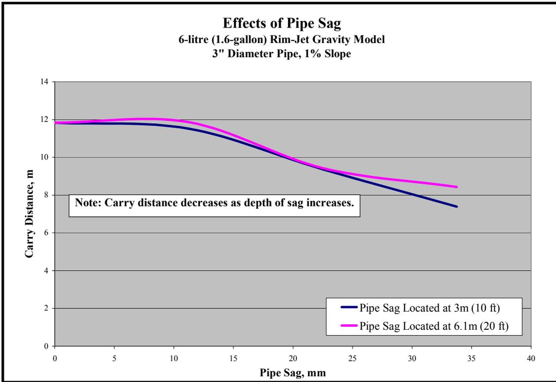
Figure 15b: Effects of Sag in Pipe Slope
