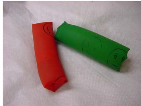
Though, as stated earlier, the comparison testing between the realistic test media used in this study and ‘Water Wigglers’ as a test media was not extensive, the results show ‘Water Wigglers’ were carried an average of 159% of the distance of the soybean media in a 3” pipe at 1% slope. Based on these limited results it does not appear that ‘Water Wigglers’ constitute a suitable test media for toilet drainline carry studies.
