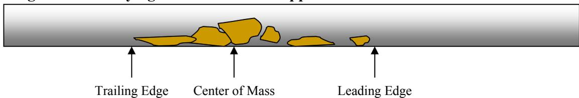
The length of waste plug sizes ranged from 12 cm (5 in) to 3.6 m (11.8 ft) with an *average* size of 63 cm (25 in) and a *median* size of 53 cm (22 in). Figure 4 illustrates the range in plug sizes (data sorted from shortest to longest length). In most cases, the second (water-only) flush tended to shorten or compact the plug length slightly. In a small number of instances it caused the plug to spread out significantly (Figure 5).
