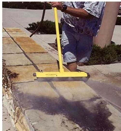
Figure 10 – 'Watermiser' Water Broom
