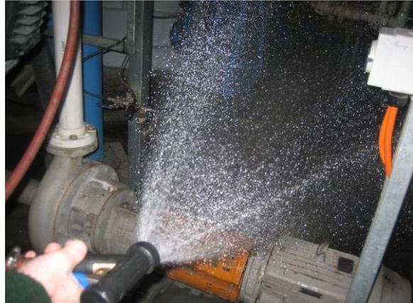
Figure 9 – A Low Flow Spray Gun 'wide' pattern
